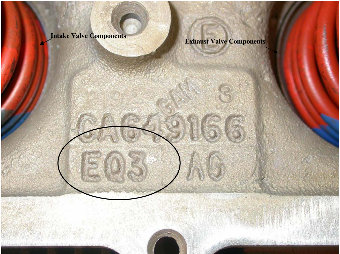
FIGURE 2 Location of EQ3 Marking in the Cylinder Head Rocker Box Overhead Area
